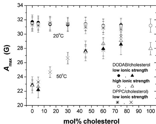
Fig. 6. Cholesterol content dependence of the outer hyperfine splitting ( $A_{max}$ ) measured on the ESR spectra of 5-PCSL in DODAB liposomes in low ( $\bullet$ ,  $\blacktriangle$ ) and high ( $\circ$ ,  $\triangle$ ) ionic strength and in DPPC in low ionic strength ( $*$ ,  $\times$ ), at 20 and 50 °C.
