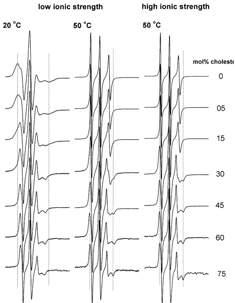
Fig. 7. ESR spectra of 16-PCSL in DODAB dispersions with different cholesterol contents, at 20 and 50 °C, the latter at low and high ionic strength. The vertical dash lines indicate the features of the ESR signal of the label in DODAB and high cholesterol amount aggregates. Total spectra width 100 G.
