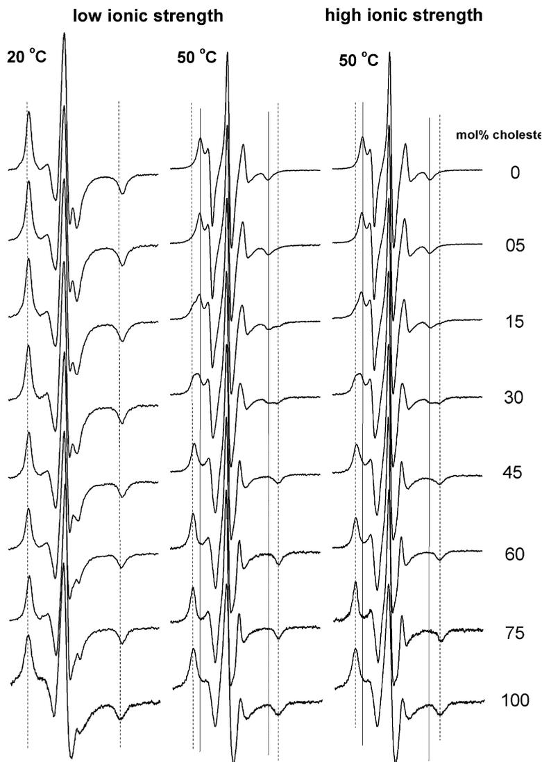
Fig. 4. ESR spectra of 5-PCSL in DODAB dispersions with different cholesterol concentrations, at 20 °C (left) and 50 °C (right), the latter at low and high ionic strength. The vertical full and dash lines indicate the features of the ESR signal of the label in DODAB and pure cholesterol aggregates, respectively. Total spectra width 100 G.
