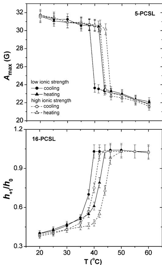
Fig. 2. Temperature dependence of the outer hyperfine splitting ( $A_{\max}$ ) measured on the 5-PCSL ESR spectra and the ratio of the low and the central field line amplitudes ( $h_{+1}/h_0$ ) measured on the 16-PCSL ESR spectra, in DODAB liposomes at low (full symbols) and high (open symbols) ionic strength, at cooling (●, ○) and heating (▲, △) procedures.
