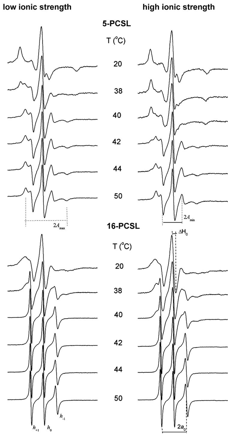
Fig. 1. ESR spectra of 5-PCSL and 16-PCSL in DODAB liposomes at low (left column) and high (right column) ionic strength, at different temperatures (cooling procedure). The outer hyperfine splitting ( $A_{\max}$ ), the three nitrogen hyperfine line amplitudes ( $h_{+1}$ ,  $h_0$  and  $h_{-1}$ , corresponding to  $m_I = +1$ , 0 and  $-1$ , respectively) and the isotropic hyperfine splitting ( $a_0$ ) are indicated. Total spectra width 100 G.
