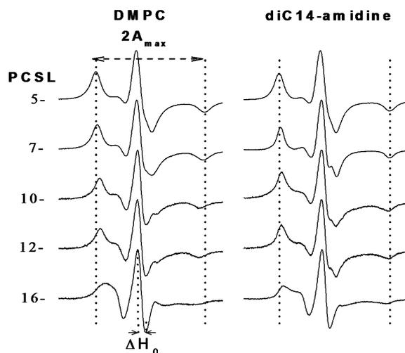
**Figure 3.** ESR spectra of 5-, 7-, 10-, 12-, and 16-PCSL incorporated in DMPC and diC14-amidine, at  $5^\circ\text{C}$ . Dotted lines indicate the positions of the outer features of the 5-PCSL spectra (outer hyperfine splitting,  $2A_{\text{max}}$ ). Total spectra width 100 G.
