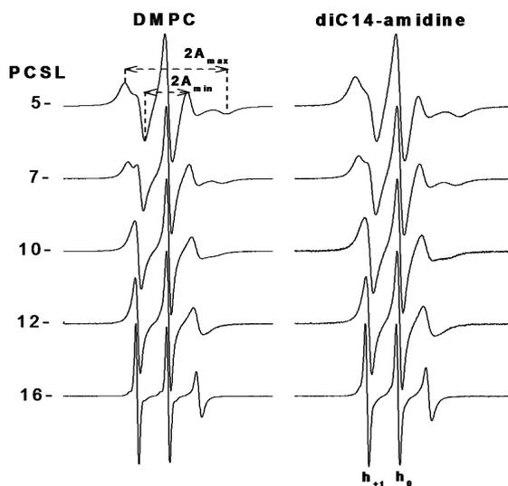
**Figure 5.** ESR spectra of 5-, 7-, 10-, 12-, and 16-PCSL incorporated in DMPC and diC14-amidine, at 40 °C. Total spectra width 100 G. Outer and inner hyperfine splittings ( $A_{\text{max}}$  and  $A_{\text{min}}$ ) are indicated, as well as the position of the  $h_{+1}$  and  $h_0$  lines.
