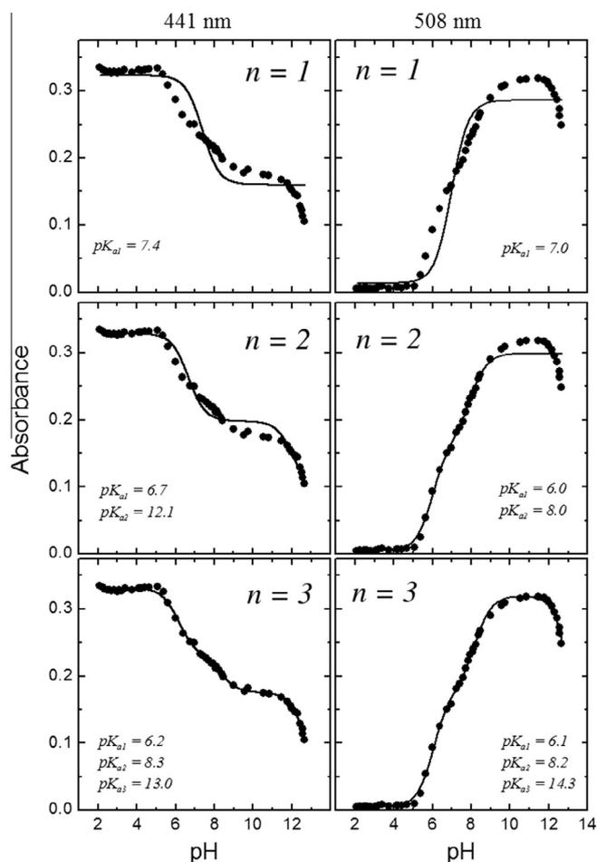
**Fig. 3.** (symbols) The Emodin absorbance at two wavelengths, 441 nm (left) and 508 nm (right), versus the apparent  $pH$  of the water–methanol mixture and (line) the best fit of the Eq. (5) with one term of the sum ( $n = 1$ , top), two term of the sum ( $n = 2$ , middle) and three terms of the sum ( $n = 3$ , bottom).
