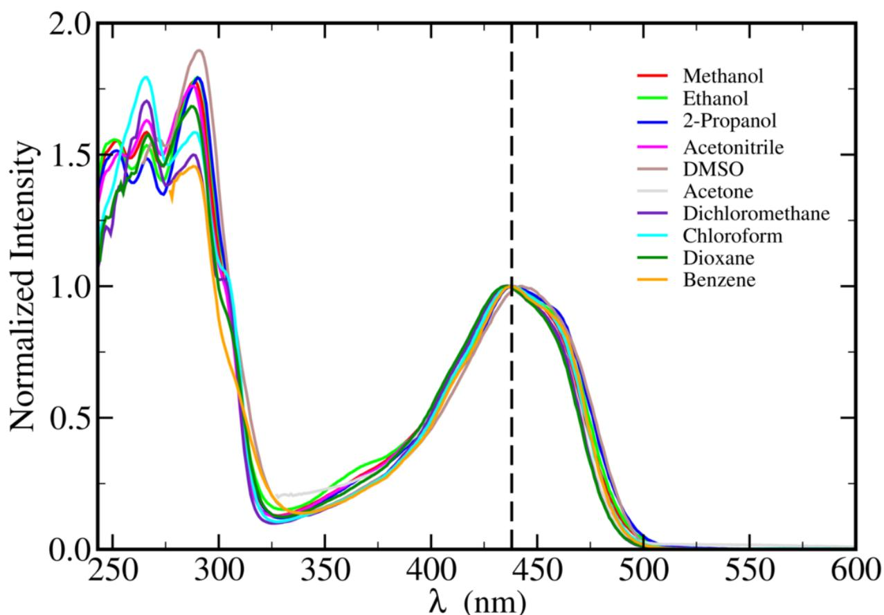
**Fig. 1:** The absorption spectra of neutral form of the Emodin (**EMH**) with concentration of 0.05 mM in different solvents. To stabilize the **EMH** in polar solvent (methanol, ethanol, 2-propanol, acetonitrile and DMSO), acid was added in the solution (1:500 v/v of HCl). The vertical dashed line shows the  $\lambda_{max}$  of the first band of **EMH** in benzene at 438 nm. The values of the  $\lambda_{max}$  and the relative intensity for all solvents are shown in Table 1.
