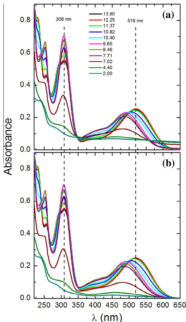
**Fig. 4.** The effect of the  $pH$  on the UV/Visible absorption spectra of the Emodin in aqueous solution at concentration of 0.025 mM, without corrections (a) and with light scattering correction (b). The vertical dashed lines show the  $\lambda_{\max}$  of the first and second bands of the Emodin in alkaline solution,  $pH > 11$ , at 519 and 308 nm, respectively.
