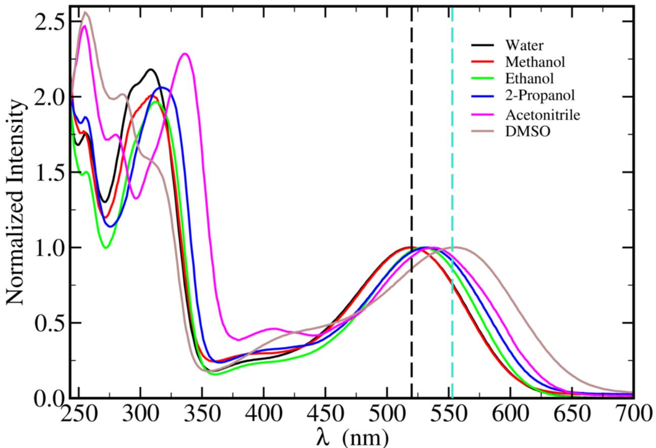
**Fig. 2:** The absorption spectra of deprotonated form of the Emodin ( $\text{EM}^-$ ) with concentration of 0.05 mM in different solvents in alkaline  $pH$  (added 17.5 mM of NaOH). The vertical dashed lines show the  $\lambda_{\text{max}}$  of the first band of  $\text{EM}^-$  in water at 519 nm and in DMSO at 553 nm. The values of the  $\lambda_{\text{max}}$  and the relative intensity for all solvents are shown in Table 1.
