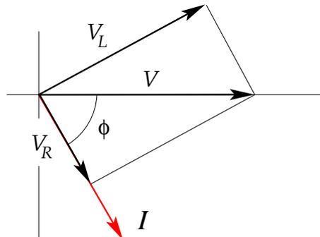
$$\begin{aligned}V &= 100 \text{ V,} \\I &= 2 \text{ A,} \\ \phi &= \frac{\pi}{3} \text{ rd.}\end{aligned}$$
